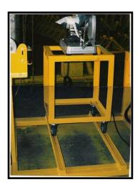
The cut off machine is used with our range of cable coiling and decoiling machines. A structural steel frame is incorporated into the main body of the coiling machine. Braked castors are fitted and travels within rails mounted to the main machine frame. A standard 220 Volt power supply is needed to power the cut off machine. This is user friendly, enhances cutting accuracy and very cheap to maintain.
